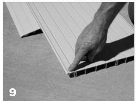
9 The hinge attachment should be flush with the end of the lid and the lid hinge is offset from the end.
