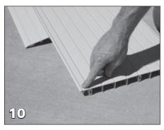
The hinge attachment (X0940) should be flush with the end of the lid and the lid hinge is offset from the end.
