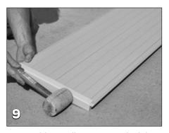
Use a rubber mallet to tap on the lid wedges on both sides of the main lid section.
