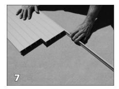
Slide the lid panels (X0048) and C-cap (X0053) together.
