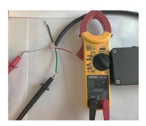
At this position the **green** and white encoder wires should be connected.
