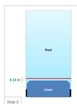
Operate cover in the **open** direction until the cover has gone 6 in. to 1 ft. past the home position.
