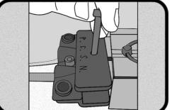
**Step 8:** Attach the new Slider to the Leading Edge Assembly. *(Fig. 8)*
