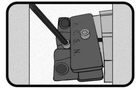
Step 4: Use a 1/8" Allen Wrench or Phillips screwdriver to remove the upper Screw on the Guide. (Fig. 4) Slide the Guide away from the Track end.
