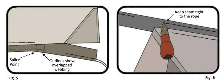
Step 7: Before cutting your stitches, sew across the webbing for three or four stitches. Cut and tie off the thread. IMPORTANT: A seam must be sewn between the end of the new rope and end of the old rope.
