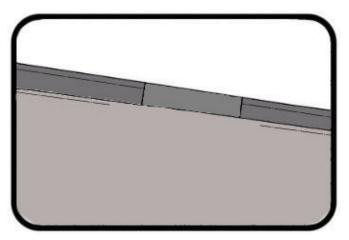
Cut webbing away from the rope within the marked area underneath the patch. This is crucial to ensure the rope will fit through the track and guides.
