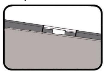
Line up the patch with the cut area so that there is no material overlapping around the rope. Begin to sew a seam next to the rope, keep the webbing as tight to the rope as possible. Once the patch is sewn to the rope you will then re-sew the web-bing to the cover, be sure to keep the webbing spaced equally. You will then sew a zig-zag seam over where the patch meets the old webbing to avoid the patch catching on the cover guide.
