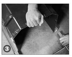
Slide polymer housing sections together and join ends tightly.
