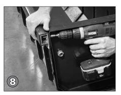
Now fasten end piece into place using eight 1" tek screws. To do this, position the end piece flush with the side wall of the housing and fasten one tek screw into each top rail as shown. All other screws should be fastened from the outside of the housing pointing in. Fasten the other box end (4, M9344) into place in the same manner on the opposite side of the housing.
