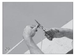
While pulling both ropes tight, use a lighter or torch to burn the rope in the location it will be cut. This will help them not fray after they have been cut. Cut the ropes so they are at least 8 ft long. Use the lighter to reburn the cut ends of the rope if needed.
