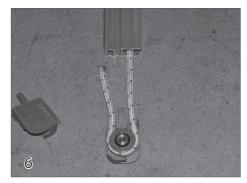
Feed the rope through the pulley cartridge assembly (13). Insert the pulley with the rope onto the end of the track.
