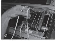
Tip: The rope for the non-motor side should be attached approximately 1 inch further down than the motor side rope depending on the width of the pool. Use the switch and operate the cover in the "Closed" position to cover the pool.
