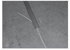
Running Ropes In The Tracks The preferred method of running the rope is to allow a short length of the rope to extend outside of the track. The portion of rope outside the track will be pulled as the rope is ran in the track.
