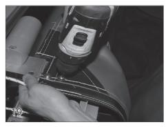
Attach the leading edge insert and slider plate to the cover by threading (2) 4-20 x 5/8" two screws (30) and the 1/4 x 5/8" washers (31) that come attached to the slider plate, through the pre-punched holes in the cover and into the slider plate. Repeat this on both sides of the cover. Use caution if using a drill to attach these screws.
