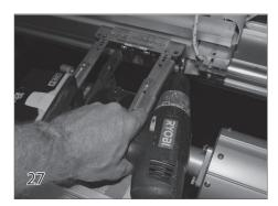
Position the fabric on the leading edge so it is in line with the edge of the rope C- channel. Pin the rope hem to the leading edge by placing a  $\#10 \times 5/8"$  pinning screw (41) in the drilled hole and through the rope hem.
