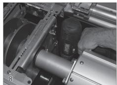
Attach the mechanism feet to the floor of the cover box. Use the mounting hardware provided.
