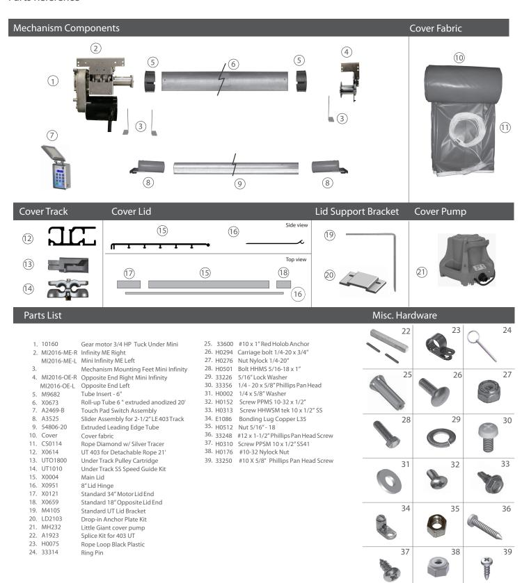
The parts list above is typical for most pools up to 16' x 32' and includes all parts necessary to install the PCS system. However, parts will vary for longer or wider pools and according to your specific order.
