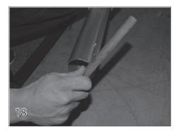
Attaching the Leading Edge Tube File the edges of the rope channel before sliding it onto the rope hem of the cover. If the leading edge tube will remain exposed, slide the tube on to the bead on the front of the cover.
