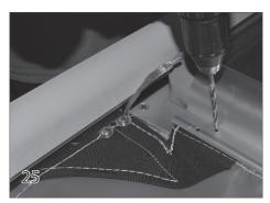
Drill a second hole using a 3/16" bit in the flat section of the leading edge just behind the rope channel. This is where a bonding lug will be attached. Do this on both ends of the leading edge tube.
