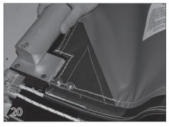
On one side of the cover, pull the rope as it comes out of the track as you feed the slider and cover into the track. Keep pulling until the slider is in the track a few inches. Having the slider on one side of the cover in the track will help with the installation of the leading edge bar.
