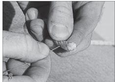
Alternate Rope Feeding Method Another common method of running rope in the track is to pierce the rope with a small piece of wire. This wire then becomes the pulling handle as you feed the rope into the end of the track. This is especially useful if retainer isn't being used and the tracks are already installed.
