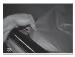
Find the center of the slack and pin directly to the tube (DO NOT FOLD THE SLACK). Repeat this step several times along the tube.
