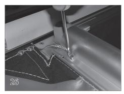
Connect the bonding wire that is attached to the front corner of the cover to the leading edge tube by first securing a bonding lug to the bar, using the 10-32 x 1" screw (33) and 10-32 nylock nut provided (40). Then, insert and tighten the bond wire in the bonding lug. Do this on both sides of the leading edge tube.
