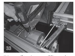
Using a self-tapping screw (33) , attach the bonding wire on both sides of the roll-up tube.
