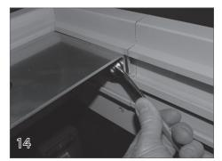
Insert the 1/4 -20 Nylock Nuts over each of the pem studs in the anchor plates. Use a 7/16" wrench to tighten the nylock nuts. Repeat installing the anchor plates and the lid lock bracket on the opposite side of the cover box.
