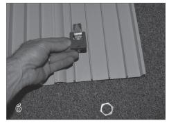
Slide the backing plate over the cam and down around the boy of the lock. The backing plate will fit between the ribs of the lid panel.
