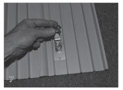
Slide the jam nut over the cam. Use channel lock pliers to tighten the jam nut down around the threads of the body so it is tight against the backing plate.
