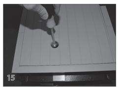
Position the fully assembled lid panels in the flush deck riser. Use a standard screw driver to twist the lid locks, which will position the lock cam in the slot of the lid lock bracket. This will lock the lid into riser.
