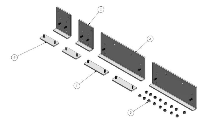
STEP 1: Attach QuickAttach plates to box perimeter extrusion.
