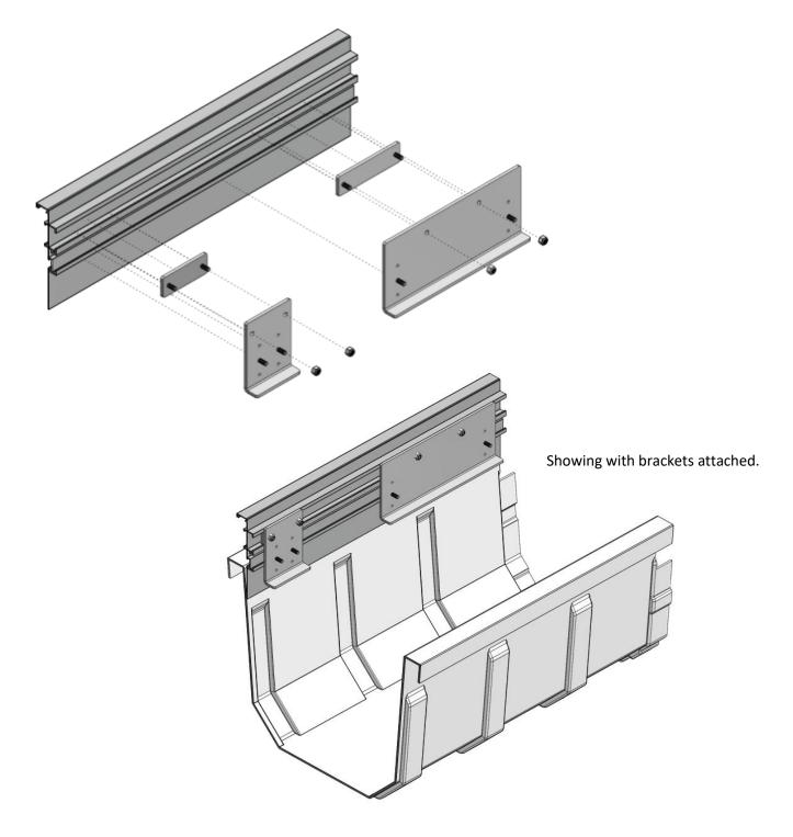
Step 2: Attach Infinity 4000 mechanism to QuickAttach brackets.
