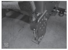
Use the 1-1/2" pan head screws (29) and anchors (16) provided to secure the motor end and non-motor end to the deck.
