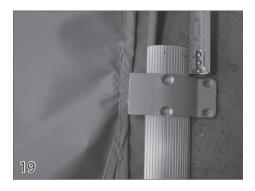
Remove the guide from the end of the track. Position the positive stop plate (36) over the track so that it is 1-1/2 inches from the end of the track.
