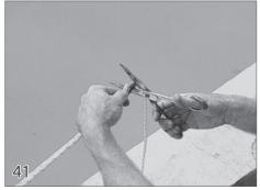
While pulling both ropes tight, use a lighter or torch to burn the rope in the location it will be cut. This will help them not fray after they have been cut. Cut the ropes so they are at least 8 feet long. Use the lighter to burn the cut ends of the rope if needed. Remember, the cover must be in the fully open position when cutting the ropes.
