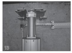
On both the motor end and non-motor end of the mechanism, measure from the cover track to the pulley. It is important that the mechanism be mounted square to the cover track.
