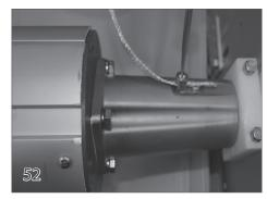
Attach the bond wire from the tail of the cover to the bonding lug (24) that is attached to the end casting.
