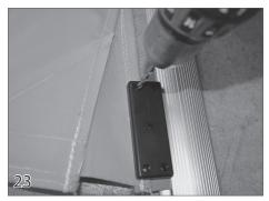
Position the top half of the positive stop (33) over the webbing of the cover. Use it as a template to drill through the holes in the positive stop and through the webbing of the cover. Remove the positive stop.
