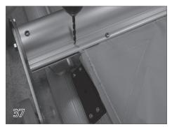
Drill a hole using a 3/16" bit in the flat section of the leading edge just behind the rope channel. This is where a bonding lug will be attached. Do this on both ends of the leading edge tube.
