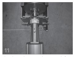
Align the mechanism on the motor side first by using a piece of rope. Extend it from the outside channel of the track to the pulley to make sure the rope will feed directly into the pulley.
