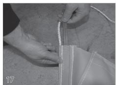
Slide the magnet (18) into the webbing with the same side facing the sensor that shut the motor off when it was passed in front of the sensor.
