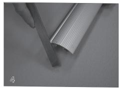
Before splicing the sections of track together, file all track ends thoroughly, rounding all edges and removing all burrs. Clean metal shavings from the track. This step is extremely important! If the track isn't filed smooth, damage can occur to the ropes and cover.
