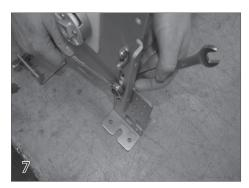
Adjust the position of the pulley brackets as needed, to spread the brackets wider to stabilize the system.
