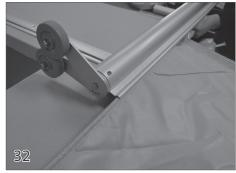
On the side of the cover that hasn't been pulled in the track yet, slide the leading edge tube on the rope hem along the front edge of the cover. Pull tight on the cover to help slide the leading edge bar onto the cover.
