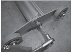
Use a 1/2" wrench, to loosen the center bolt of the wheel assembly. Repeat steps 27 - 29 on the opposite side of the cover.
