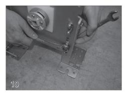
Use a 1/2" wrench to tighten the nylock nuts.
