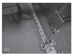
With the cover in the fully closed positon, measure back 6-1/2 inches from the guide and place a mark on the webbing.
