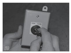
Run the key switch in the open position to roll the cover up on the roll-up tube. Check the cover to be sure it rolls up evenly. Run the cover 6-10 times to make sure it opens and closes evenly. The cover fabric installation is now complete.
