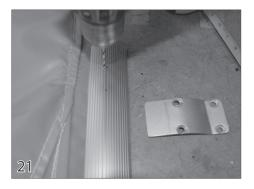
Use a 1/4" drill bit to drill the holes in the track.
