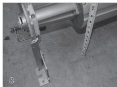
Install the roll-up tube as high as possible to prevent the cover from rubbing on the deck as the cover rolls up.
