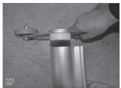
Insert the wheel assembly (6) into the leading edge.
