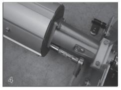
With the motor end turned upside down, attach the cone on the motor end using the same bolts (37) and washers (38). Tighten the bolts using a 9/16" wrench or ratchet.
