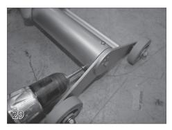
Insert screws (28) into each hole to connect the leading edge to the wheel assembly.
