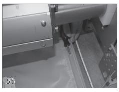
Insert a screw driver through the slit in the webbing to create the pocket for the magnet.
