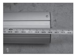
To determine if the cover system was ordered correctly for the pool, the length of the roll-up tube should be 6 inches shorter than the track space. For example, for an 16 ft track space, the correct length of roll-up tube is 15 ft 6 in.
