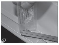
Apply the supplied grease to the magnet. This will help it slide in the webbing easier.
