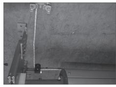
On the non-motor end, run the rope around the pulley and out the backside of the pulley assembly. Pull this rope along the back of the mechanism to the motor end pulley assembly. Be sure to route the rope in front of the lid brackets.
