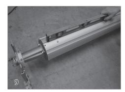
With the mechanism and tube assembled, check the roll-up tube for level. If the deck isn't level, the distance from the deck to the tube should be the same on both ends of the tube.
