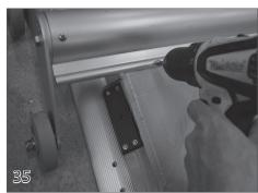
Use a 5/32" bit to drill through the C-channel of the leading edge. Do not drill through the cover. Insert a #10 x 1/2" screw (26) to pin the cover to the leading edge.
