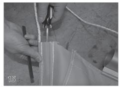
On the front corner of the cover, that is on the same side as the motor, insert a screw driver into the end of the webbing to open it up and create a pocket.
