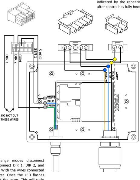
**NOTE:** To change modes disconnect power, then connect DIR 1, DIR 2, and COM together. With the wires connected reconnect power. Once the LED flashes blue disconnect the wires. This will cycle through the modes.
