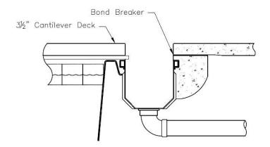
Use control joint around housing if cracking is a concern
