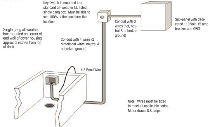
**OPTIONS** - Coverstar has several different wiring options that includes limit switches, wireless remote control, water feature shutoffs etc. Contact your Coverstar distributor for details. **Note:** Builder is responsible to bring proper electric lines, conduit and bonding to the mechanism.
