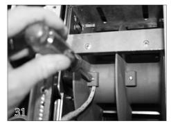
Bring the ropes back to the mechanism. Attach the ropes to the rope reel by inserting the ropes through the center of the lugs and tighten the set screws firmly into the ropes. Some prefer to tie a knot at the end of the rope.
