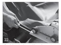
Feed the wheel assembly and cover into the track. The slider on the front of the wheel assembly will lock into the track.
