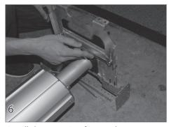
Install the mounting feet on the non-motor end using the bolts (43) and lock washers (52) provided. The top of the pulley bracket on the non-motor end should be flush with the top of the track.
