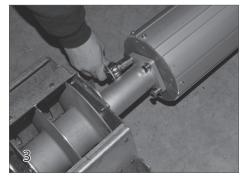
With the motor end turned upside down, attach the cone to the motor end of the mechanism using the 3/8" x 1-1/4" bolts (50) and lock washers (44) provided. Tighten these bolts with a 9/16" wrench.
