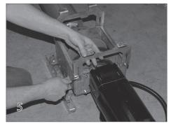
With the motor end positioned upside down, install the mounting feet using the bolts (43) and lock washers (52) provided.
