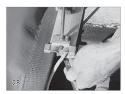
Place a bonding wire lug (33) on top of the guide feed and secure with a 10-32 1-3/8" screw (48) and nylock nut (38).
