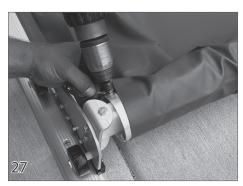
Connect the bonding wire that is attached to the front corner of the cover to the leading edge bar using a tek screw (49). Be sure the screw doesn't interfere with the leading edge insert.
