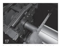
Raise the pulley bracket so it is level with the top of the cover track. Center the non-motor side front to back in the housing.
