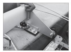
Attach the rope tab to the wheel assembly.
