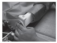
Place the nylon leading edge inserts into the ends of the leading edge tube. Make sure they can slide freely inside the leading edge tube.
