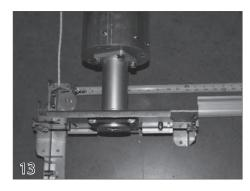
On both the motor end and non-motor end of the mechanism, measure from the cover track to the pulley. It is important that the mechanism be mounted square to the cover track.
