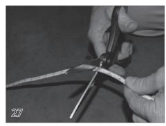
Pull both ropes until the leading edge just moves on each side, cut the longer rope to the same length as the shorter rope while tight. These ropes should be at least 8 ft long. Use a lighter or torch to burn the ends of the rope. In most cases you will only need to cut one rope.
