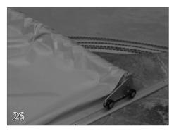
Pull the cover back until the cover is in the tracks equally on both sides. Pull the ropes tight as they come off the pulleys on the mechanism to eliminate the slack in the rope.
