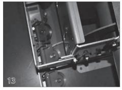
Bend a curve into the end of the wire and pull it back just until it is in the middle of the pulley. Now push the wire back until it comes out the side of the third pulley.
