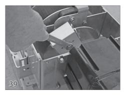
If further adjustment is needed, rotate the torque limiter brake arm to position the second brake bolt and tighten the second brake bolt 1/2 turn.
