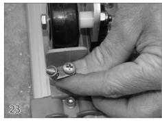
Place a bonding lug (16) on top of the guide feed. Insert a 10-32 x 1-5/8 screw (34) through the lug, guide feed, and track. Install a 10-32 nylock nut (21) and tighten with a 3/8" wrench.
