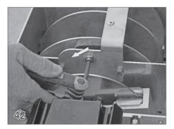
To tighten the brake, use an allen wrench to turn the set screw inside the jam nut in the clockwise direction.
