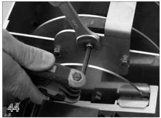
After adjusting the set screw, retighten the jam nut while holding the set screw with an allen wrench. There's a corresponding brake on the opposite side of the rope reel. Adjust both brakes equally.
