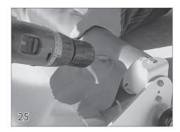
Position the fabric on the leading edge so it is in line with the leading edge support bracket. Secure with a tek screw (24) on the back side of the leading edge. Be sure the screw does not interfere with the leading edge insert.
