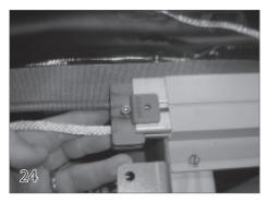
Slide the guide feed onto the track with the flange inserted in the slider channel.
