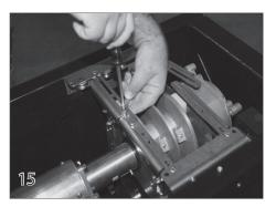
On the motor <u>and</u> non-motor side, use the half inch screws (26) and nylock nuts (27) provided and secure the cross braces together.
