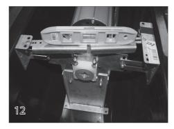
With the brackets on the non-motor end in position, place a small level across the brackets to make sure they are level with the bottom of the track. Tighten the nylock nuts on the adjustable brackets.
