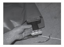
Insert the leading edge inserts (9) into the leading edge tube. When using the 1" or 2-1/2" leading edge bars, make sure the end cap is in place before inserting the leading edge insert.
