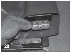
Attach the leading edge insert to the slider by inserting the a screw (39) from the bottom of the slider. The screw will go through a punched hole in the cover, then into the leading edge insert.
