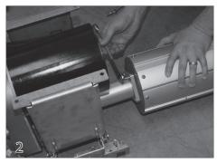
Attach the roll-up tube to the motor end of the mechanism using the  $3/8" \times 1-1/4"$  bolts (34) and lock washers (35) provided.
