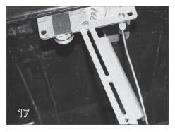
Make the same connection with the #8 copper bond wire (36) that is in the cover box on the non-motor end of the mechanism.
