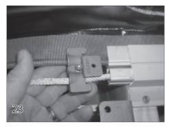
Turn guide feed back to closed over the rope and webbing then tighten the allen bolt.
