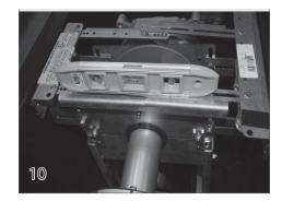
With the brackets in position, place a small level across them to make sure they are level. Tighten the four nuts on the adjustable motor end brackets.
