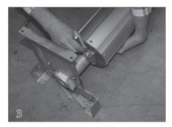
Attach the roll-up tube to the non-motor end of the mechanism using the  $3/8" \times 1-1/4"$  bolts (34) and lock washers (35) provided.
