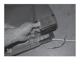
On the opposite side of the cover that isn't in the track, insert the leading edge tube (10) into the loop of the cover.
