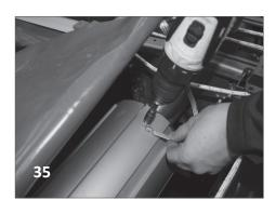
Using a self-tapping screw (30), attach the bonding wire on both sides of the roll-up
