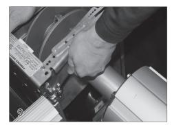
Loosen the four nylock nuts on the pulley brackets. Raise the pulley bracket assembly so it is level with the bottom of the track.
