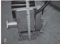
Attach the mechanism feet to the mechanism approximately 1 inch less than the distance from the bottom of the cover box to the top of the track/retainer. Use a 7/16" ratchet to tighten bolts.
