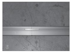
Continue tapping the end of the track until the two sections of track are tight together so there is not a gap from one track to the next.
