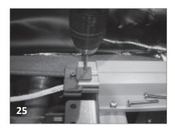
Drill a hole through the guide feed into the track for the attachment bolt.
