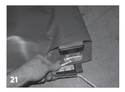
Tighten the nut (27) all the way down, then loosed ½ turn to allow movement between the slider and the leading edge insert. Repeat the installation of the leading edge insert on the other side of the cover.
