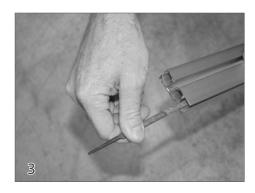
Before splicing the sections of track together, file all track ends thoroughly, rounding all edges and removing all burrs. This step is extremely important!
