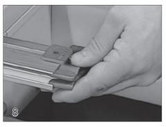
Using a 5/32" allen wrench, loosen the screw on the top of the guide feed (15). Insert the guide feed on the end of the track that will extend into the cover box.
