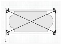
Position the cover track along both sides of the pool. The lengths, widths and diagonal measurements <u>must</u> be equal to each other for the automatic cover system to operate properly. Mark where the center of the track will be on the pool deck.
