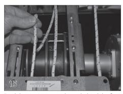
Feed the non-motor end rope behind the first and second and third horizontal pulleys.
