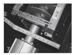
Center the tube in the cover box. Tip: If the pool is not square, square up the mechanism with the track.
