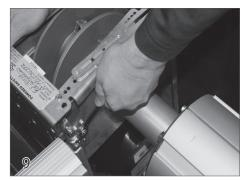
Loosen the four nylock nuts on the pulley brackets. Raise the pulley bracket assembly so it is level with the bottom of the track.
