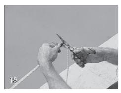
While pulling both ropes tight, use a lighter or torch to burn the rope in the location it will be cut. This will help them not fray after they have been cut. Cut the ropes so they are at least 8 ft long. Use the lighter to reburn the cut ends of the rope if needed.
