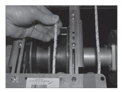
On the motor end, feed the rope around the first and second horizontal pulleys on the back wall of the cover box.
