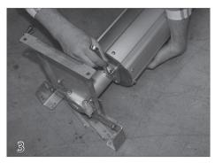
Attach the roll-up tube to the non-motor end of the mechanism using the  $3/8" \times 1-1/4"$  bolts (44) and lock washers (50) provided.
