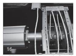
Pull the rope around the vertical pulley on the front wall of the cover box.
