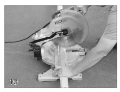
Cut the track at the mechanism end to the proper length using a miter saw. It is important to have square cuts on the track. Note: Always wear safety goggles when using powered equipment.
