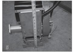
Attach the mechanism feet to the mechanism approximately 1 inch less than the distance from the bottom of the cover box to the top of the track/retainer. Use a 7/16 inch ratchet to tighten bolts.
