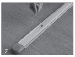
Feed the rope into the back channel then pull the rope down the back side of the track toward the cover housing.
