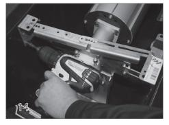
Anchor the non-motor side of the mechanism into the cover box in as many places as possible. Use the appropriate screws and anchors depending on the type of cover box being used.
