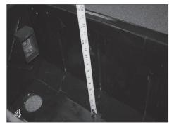
To attach the feet, first measure the distance from the bottom of the cover box to the bottom of the track.
