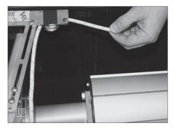
On the non-motor end, feed the rope around the pulley of the non-motor end pulley bracket. Pull the rope through to the motor end.
