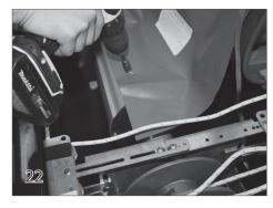
Using a self-tapping screw (32), line the cover up straight as it comes out of the track and pin the cover to the roll-up tube on both sides.
