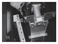
Loosen the bolts on the adjustable brackets on the non-motor end of the mechanism. Spread the pulley brackets outward against the walls of the cover box.
