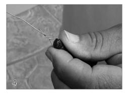
Running Ropes Through the tracks The preferred method of running the rope is to pierce the rope with a 1' length of wire and use it as a handle to feed the rope through the track.
