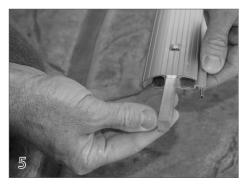
Tap the spring pin (46) into the round splice channel. Slide the center splice (45) into the center channel.
