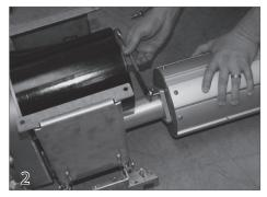
Attach the roll-up tube to the motor end of the mechanism using the  $3/8" \times 1-1/4"$  bolts (44) and lock washers (50) provided.
