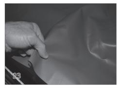
Find the center of the slack and pin directly to the tube (DO NOT FOLD THE SLACK). Repeat this step several times along the tube. This will help to distribute the slack across the roll-up tube evenly.
