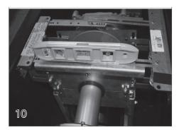
With the brackets in position, place a small level across them to make sure they are level. Tighten the four nuts on the adjustable motor end brackets.
