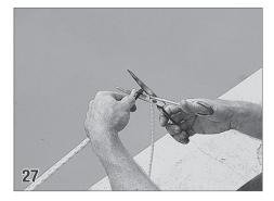
While pulling both ropes tight, use a lighter or torch to burn the ends of the rope. Cut the ropes so they are the same length. These ropes should be at least 8 feet long. Use a lighter or torch to burn the ends of the rope to keep the rope from fraying. In some cases you will only need to cut one rope.
