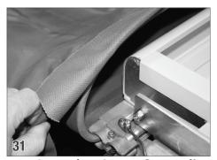
Attaching the Cover & Bonding Wire Make sure the webbing continues straight as it travels from the track to the rollup tube. Attach the cover to the roll-up tube using tek screws (32). The first screw on each end of the tube needs to be 3 inches from the end of the tube. As the cover rolls up on the tube, the webbing should roll up completely off the tube.
