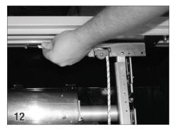
On the non-motor end, run the rope from the back channel of the track around the pulley.
