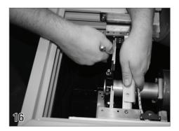
Now loosen the bolts and spread the pulley brackets at the non-motor end making sure they are also level. Raise the pulley bracket so it is flush with the top of the encapsulation.
