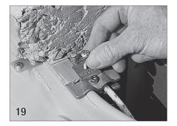
Place a guide feed over the end of the track, place a bonding lug (25) on top of the guide feed. Insert a  $10-32 \times 1-3/4''$  screw (42) through the lug and guide feed.
