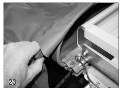
Run #8 copper bond wire (38) from the lug on each guide feed to the lugs on each mechanism end.
