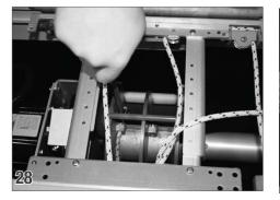
Bring the ropes back to the mechanism. Slide the rope through the rope lug on the rope reel. Secure the ropes to the reel by tightening down the set screws in each lug.
