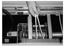
If both ropes are the same length, and the cover doesn't close squarely, shorten the rope for the side of the cover that doesn't close all the way. The amount that the rope is shortened is equal to the amount distance that the cover needed to travel to close all the way. While holding the rope, run the switch in the cover position.
