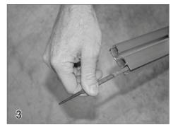
Before splicing the sections of track together, file all track ends thoroughly, rounding all edges and removing all burrs. This step is extremely important!
