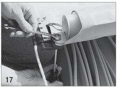
Secure the leading edge support bracket to the slider by placing the  $10-32 \times 1''$  (41) screw up through the slider, the hole in the front corner of the cover, and through the support bracket. Tighten completely using 10-32 nylock (29), then back the nut off 1/2 turn.
