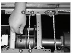
Run the non-motor end rope behind the motor end rope as it passes behind pulleys #1 and #2 and around pulley #3. Continue pulling the rope to the front side of the mechanism. Run the rope around pulley #5 with the rope coming off the bottom of the pulley. Pull all the excess rope through and lay it on the deck in front of the mechanism.
