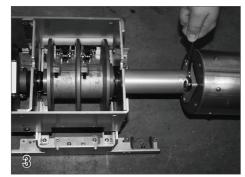
With the motor end turned upside down, attach the cone on the motor end using the same bolts (36) and washers (37). Tighten the bolts using a 9/16'' wrench.
