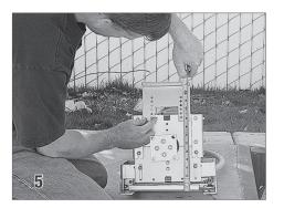
Position the mechanism with the pulley brackets on the bottom. Install the feet on the mechanism using the carriage bolts (35) and nylock nuts (40) provided. Install the feet so the top of the mechanism will be flush with the top of the encapsulation.
