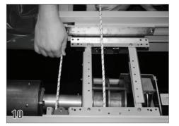
Align the mechanism on the motor side first by using a straight edge or a piece of rope and extending it from the back side of the cover track to the pulley to make sure the rope is running straight into pulley #1.
