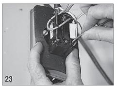
Insert the **RED DIRECTIONAL WIRE** into terminal B1, and tighten the screw.
