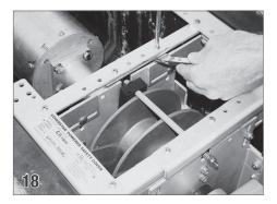
On the motor and non-motor side, use a 3/16" bit and drill through the cross braces. To secure, use the half inch screws (28) and nylock nuts (29) provided and bolt the cross braces together in two places on each cross bracket.
