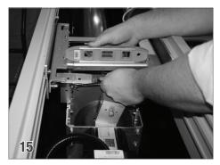
With the brackets in position, level the pulley brackets. Tighten the four nuts on the adjustable brackets.
