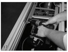
Anchoring the Pulley Brackets Anchor the motor and non-motor end brackets into the housing in as many places as possible.
