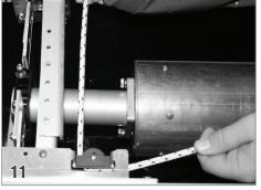
On the non-motor end, make sure the rope will travel straight from the track to the pulley. It is important that the rollup tube be centered between the cover tracks.
