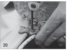
Use a 5/32" allen wrench to tighten the screw that connects the two sections of guide feed together.
