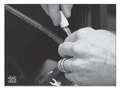
Attach the other leg from the indicator light and the **BLUE DIRECTIONAL WIRE** into terminal A1, and tighten the screw.
