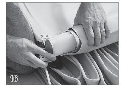
Place the nylon leading edge inserts (10) into the ends of the leading edge tube. Make sure they can slide freely inside the leading edge tube. The grooves in the leading edge insert should line up with the tongues in the leading edge tube.
