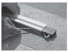
Now, feed the rope through the pulley assembly. Insert the pulley into the end of the track.
