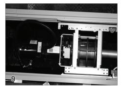
Position the mechanism in the housing so that the roll-up tube is centered in the housing front to back.
