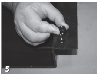
5 Loosely thread the thumb screws into the t nuts that are pressed into the lid form tray.
